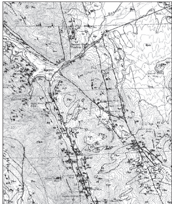
Figure 3. Portion of the unpublished Geologic map of the Julian Quadrangle by Victoria Todd. Kgm: Tonalite of Granite Mountain; Jhc: Harper Creek Gneiss; Kcr: granodiorite of Cuyamaca Reservoir; Jtrm; Julian Schist.
