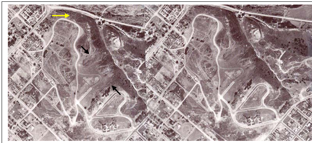
Figure 4. San Diego County 1928 photographs of Presidio Park area. Black arrows point to northeast trending fault scarps bounding the Presidio Park Graben. Yellow arrow points to possible right-lateral offset of valley wall. Geologic map Figure 1 shows a pressure ridge and possible closed drainage south of the road below the yellow arrow that may be evidence of a landslide or an active fault.
