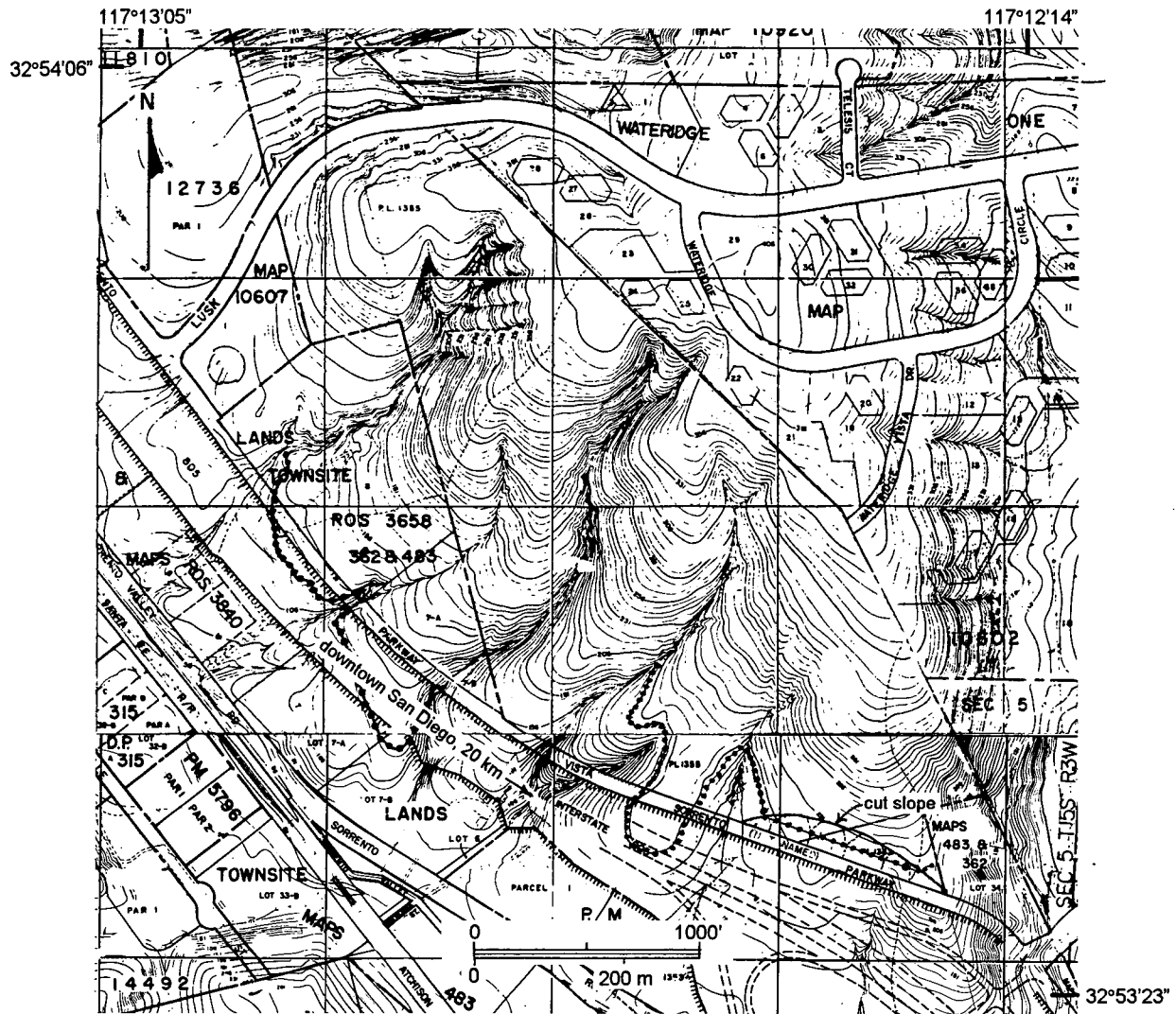
Figure 7. Vista Sorrento Parkway BPS locality. Two BPS (dotted lines) are present in this location within the Eocene Scripps Formation and Ardath Shale. Note relatively uniform slope contours and lack of distinctive landslide morphology. Interval between bold contours is 25 ft.
