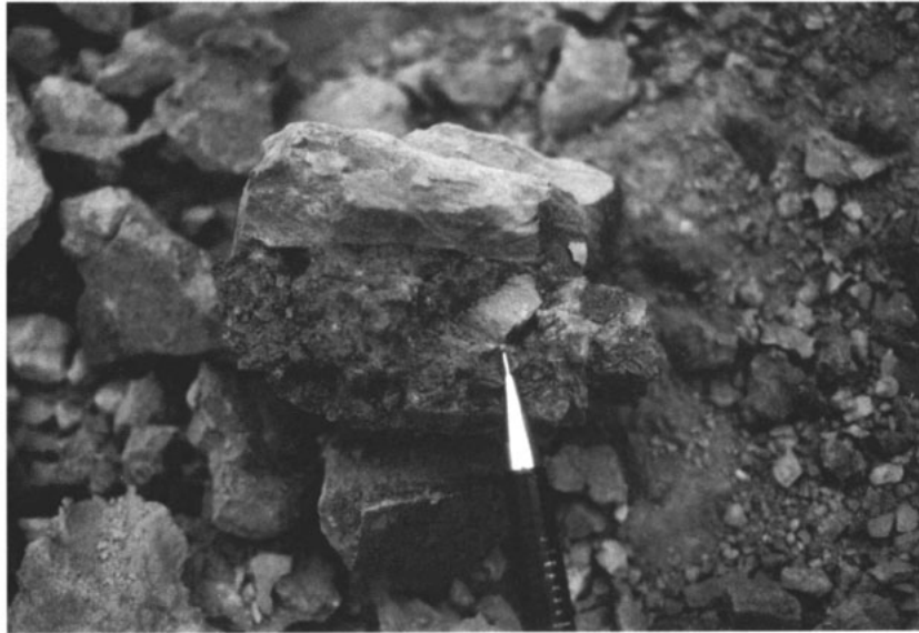
Figure 9. Approximately 2.5 cm thick gouge zone of Vista Sorrento Parkway BPS. Note the angular clast of siltstone at tip of pencil.
