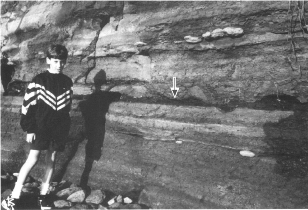
Figure 13. BPS (arrow) near base of sea-cliff, Leucadia, California. Note pinch-and-swell nature of gouge zone suggesting squeezing of clay bed and plastic flow.
